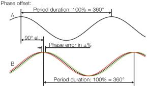
El. phase offset:  $90^{\circ} \pm max$ . phase error 7,5% of a period duration
