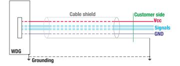
L2/L3, T3: Cable shield connected to encoder housing. Encoder housing not earthed separately.
