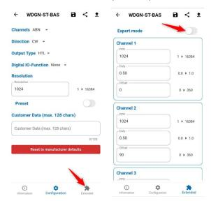
When you have set all your parameters as desired, tap and then tap 1, to transmit the configuration to the encoder.
