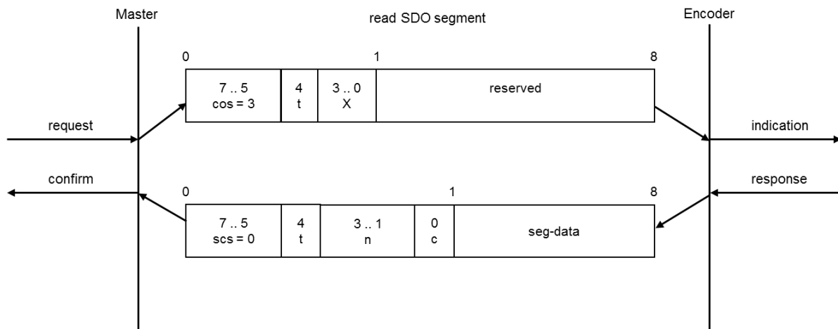
Figure 8.5: read SDO segment
