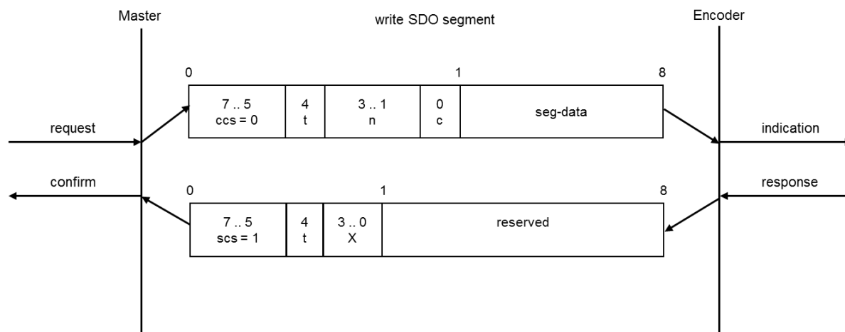
Figure 8.8: write SDO segment
