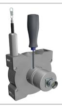
By tightening (approx. 2 Nm) the inner radial screw with a 2.5 mm hex wrench the encoder shaft will be clamped to the sensor mechanics and secured from twisting.
